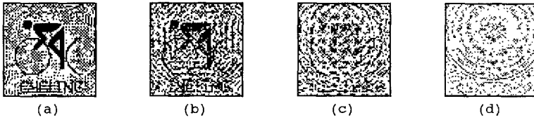
Figure 4. Effect of poor sampling of the receiver data on the reconstructed image. The complete receiver data contains 128 \times 128 points. The figure shows the reconstructed images using different sampling rates. The unknown samples are set to zero. The figure shows the reconstructed image using (a) 64 \times 64 points on the receiver plane, (b) 32 \times 32 points on the receiver plane, (c) 16 \times 16 points on the receiver plane, (d) 8 \times 8 points on the receiver plane. In all cases only one frame of data is used for reconstruction, and finite support constraint is used as the a priori knowledge. Note the degradation when the number of sampling points decreases.
