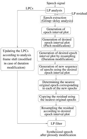
Fig. 4. Block diagram for prosody modification.
