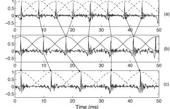
Fig. 10. Pitch period modification using LP-PSOLA method. (a) Modified residual signal using LP-PSOLA method for pitch period modification factor  $\alpha = 0.75$ . (b) LP residual for a segment of voiced speech. (c) Modified residual signal using LP-PSOLA method for pitch period modification factor  $\alpha = 1.33$ .
