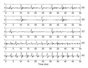
Fig. 11. (a) LP residual for a segment of voiced speech. (b) Modified LP residual signal using LP-PSOLA method for pitch period modification factor  $\alpha = 2$ . (c) Modified LP residual signal using epoch-based method for  $\alpha = 2$ . (d) Modified LP residual signal using LP-PSOLA method for  $\alpha = 0.5$ . (e) Modified LP residual signal using epoch-based method for  $\alpha = 0.5$ .
