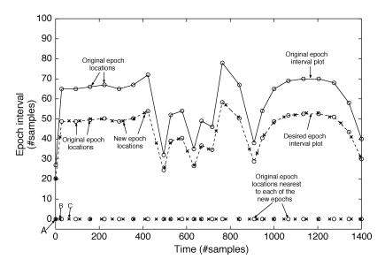
Fig. 5. Generation of new sequence of epochs for the modification of pitch period by a factor  $\alpha = 0.75$ .
