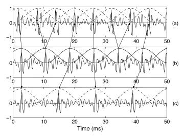
Fig. 1. Pitch period modification using TD-PSOLA method. (a) Modified speech signal using TD-PSOLA method for pitch period modification factor  $\alpha = 0.75$ . (b) A segment of voiced speech (original). (c) Modified speech signal using TD-PSOLA method for pitch period modification factor  $\alpha = 1.5$ .
