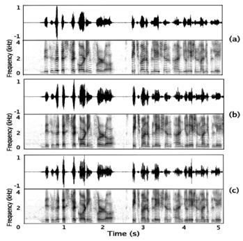
Fig. 9. Speech signal and its narrowband spectrogram for the utterance "*This* is a test recording for pitch manipulation and duration manipulation." (a) Pitch period modification factor  $\alpha = 0.66$ , (b) original, and (c) pitch period modification factor  $\alpha = 1.33$ .
