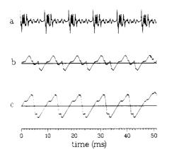
Fig. 9. Phase slope function for the output of an all-pole model excited by the periodic impulses sequence of Fig. 8(a): (a) Output of an all-pole model excited by a periodic impulses sequence; (b) phase slope function for a window size of 6.4 ms; (c) phase slope function for a window size of 12.8 ms.
