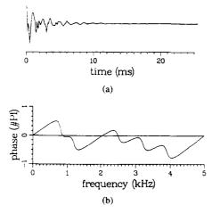
Fig. 1. (a) Impulse response of a minimum phase (five resonator) system and (b) its phase spectrum.
