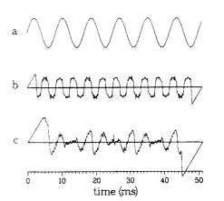
Fig. 12. Phase slope function for a sinusoidal sequence: (a) Sinusoidal sequence; (b) phase slope function for a window size of 6.4 ms; (c) phase slope function for a window size of 12.8 ms.
