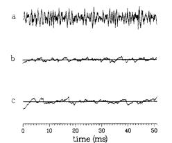
Fig. 11. Phase slope function for an all-pole model excited by a random noise sequence: (a) Output of an all-pole model excited by a random noise sequence; (b) phase slope function for a window size of 6.4 ms; (c) phase slope function for a window size of 12.8 ms.
