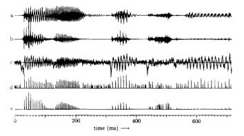
Fig. 14. Illustration of the method for a portion of the utterance for the sentence "ANY DICTIONAry will give ..." by a male speaker: (a) Speech signal; (b) linear prediction residual; (c) phase slope function for the linear prediction residual signal; (d) confidence plot for the positive zero-crossing instants of the smoothed phase slope plot; (e) gain plot showing the strengths of the impulses at the significant instants.
