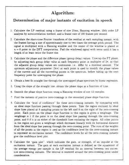
Fig. 6. Algorithm for determination of major instants of excitation.
