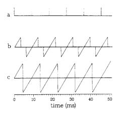
Fig. 7. Phase slope function for a periodic impulse sequence; (a) Periodic impulse sequence; (b) phase slope function for a window size of 6.4 ms; (c) phase slope function for a window size of 12.8 ms.
