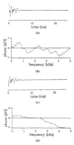
Fig. 2. Effects of truncation on the phase characteristics of the minimum phase signal of Fig. 1: (a) Right truncated signal of Fig. 1(a); (b) phase spectrum of the signal in (a); (c) left truncated signal of Fig. 1(a); (d) phase spectrum of the signal in (c).
