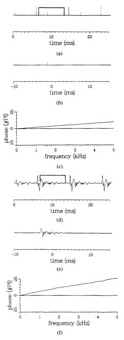
Fig. 3. Rectangular window of 6.5 ms, centered at t = 10 ms, is used: (a) Periodic impulses sequence; (b) windowed segment of (a) with the center of window at t = 0; (c) phase spectrum of the signal in (b); (d) response of an all-pole filter for the periodic sequence in (a); (e) windowed segment of (d) with the center of the window at t = 0; (f) phase spectrum of signal in (e).
