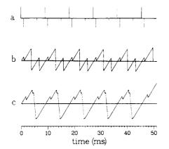
Fig. 8. Phase slope function for a periodic impulses sequence: (a) Periodic impulses sequence; (b) phase slope function for a window size of 6.4 ms; (c) phase slope function for a window size of 12.8 ms.
