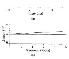
Fig. 4. (a) Signal of Fig. 3(e) multiplied by a Hanning window, and (b) phase spectrum of the signal in (a). The average slope is equal to the average slope in Fig. 3(c). Therefore, it is now dictated by the excitation rather than the window, which was the case in Fig. 3(f).
