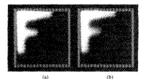
Fig. 5. Image reconstruction from FT magnitude: approximate minimum phase signal. (a) Original. (b) Minimum phase equivalent image from FT magnitude.
