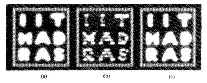
Fig. 6. Image reconstruction from FT phase. (a) Original. (b) Minimum phase equivalent image from FT phase. (c) Iterative image reconstruction from FT phase.
