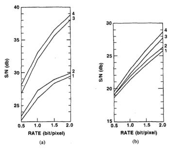
Fig. 1. Simulation results for (a) "Cronkite" and (b) "Plant." Curves 1 and 2: nonuniform Gaussian quantizer. Curves 3 and 4: pdf-optimized quantizer. Curves 1 and 3: rate-distortion theoretic approach. Curves 2 and 4: computational approach.
