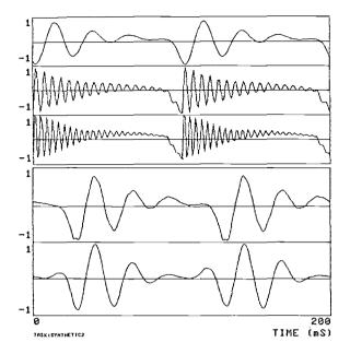
FIG. 4 Simulated data and extracted first formant wavefrom. From top to bottom  $F_1$ : 400 Hz, ±1  $F_2$ : 1800 Hz, ±0.5  $F_3$ : 2570 Hz, ±0.025  $F_1 + F_2 + F_3$ Estimated  $F_1$
