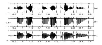
Figure 4: Continuous speech of a male voice for the utterance "She has left for a great party today" (http://archives.limsi.fr/VOQUAL/voicematerial.html). (a) speech signal, (b) differenced EGG signal, and (c) filtered signal
