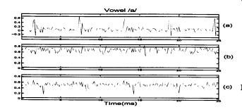
Fig. 5. For a segment of vowel /a/, (a) Normalized LP residual, (b) Frame confidences for genuine speaker, and (c) Frame confidences for an impostor speaker.
