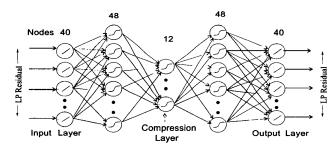
Fig. 3. Structure of AANN Model used for capturing speakerspecific source information
