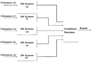
Fig. 10. Block diagram of online speaker verification system.
