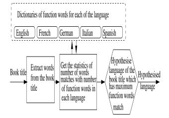
Fig. 1. Block diagram of the system for automatic language identification.
