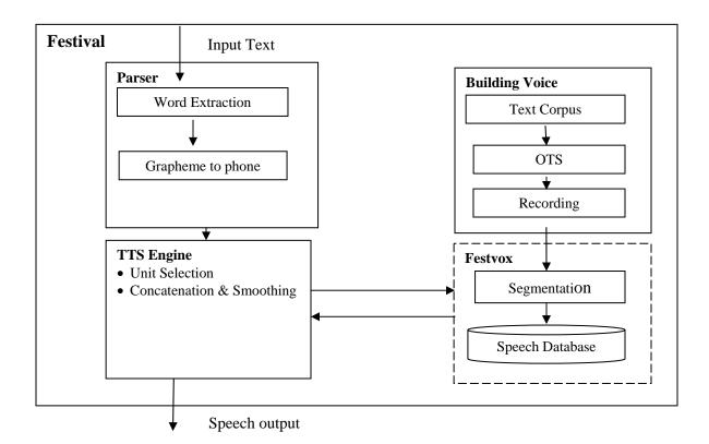
Figure 2. System architecture of Bengali TTS
