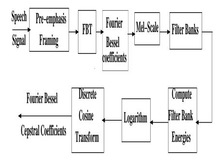
**Fig. 4.** Block diagram illustrating the steps involved in the computation of the Fourier Bessel cepstral coefficients (FBCC).
