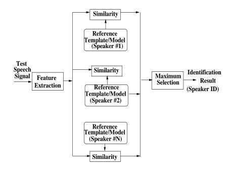
Fig. 1. Basic flow diagram of a closed-set speaker identification system.
