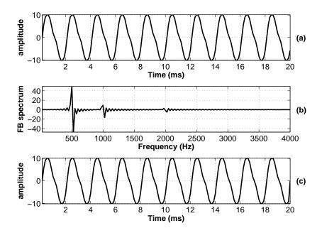
**Fig. 3.** Multicomponent signal (a) original signal (b) FB coefficients (c) Reconstruction of the original signal using fewer number of FB coefficients.
